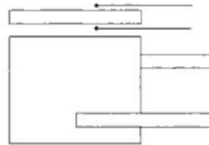
(e) Wafer (Typical dimension 1.25 mm to 15 mm × 0.3 mm thickness)
