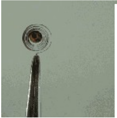
Figure 7-3. Bimetallic dial thermometer
